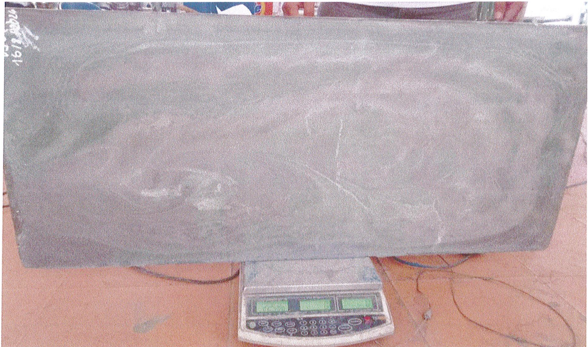
Figure 4. The weight of lightweight concrete panel
