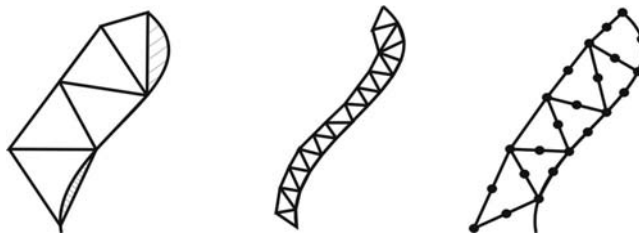
FIGURE 9.4 Geometrical discretization error.
